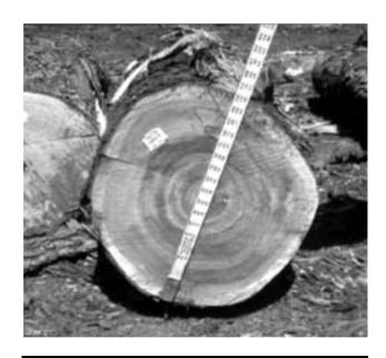
**Scaled Logs** — As logs arrive at the Harden factory, they are rated by size, quality, curvature, knots and other quality-indicators.
