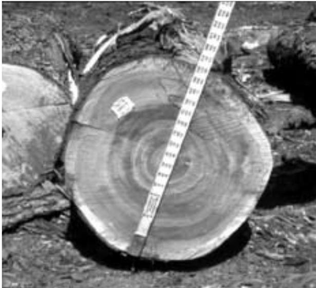
*Scaled Logs* — As logs arrive at the Harden factory, they are rated by size, quality, curvature, knots and other quality-indicators.
